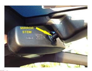
**STEP 5 -** While sitting in the passenger seat, place the mount over the mirror stem. Tighten the CLAMP SCREW until the mount starts to clamp onto the mirror stem. Position the mount as far forward as it will go and paralell to the bottom of the mirror before fully tightening.
