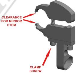
**STEP 3** - The BODY ASSEMBLY must be removed to gain access to the CLAMP SCREW. Remove the two socket head screws as shown above. Be sure to remove the lock washer with the top screw along with the lock washer and flat washer with the bottom screw.
